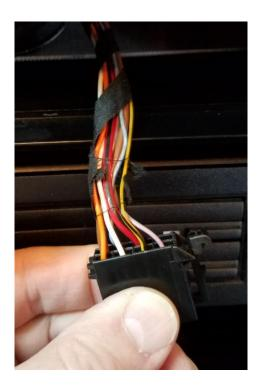
b. Locate ORANGE (+) wire, install red T-Tap as shown close to plug:
