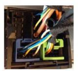
Fig. 13 Factory Quadlock Plug and sub-plugs
