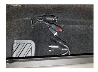
e. Either remove CD Changer and store, or put back in as removed, leaving wires disconnected.
