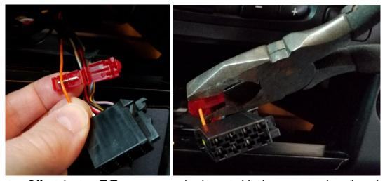
**Note:** Offset the two T-Taps – so one is closer to black connector than the other.
