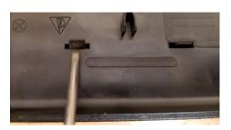
e. <u>OPTIONAL: DRILL HOLE FOR BT RECEIVER TO BE LOCATED INSIDE STORAGE SHELF.</u>
